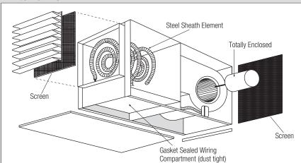
in high rise buildings. Ducted heated air supply for garage ventilation systems.
