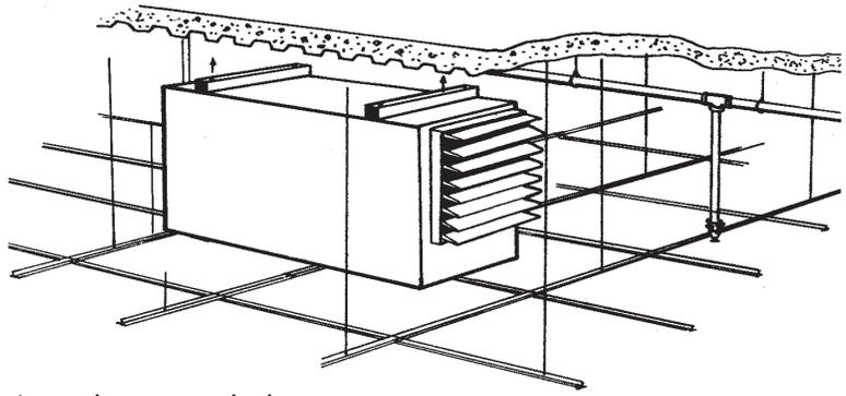
It is also suitable for use as a special purpose unit heater where the environmental requirements are dirty, dusty, moist or mildly corrosive.
