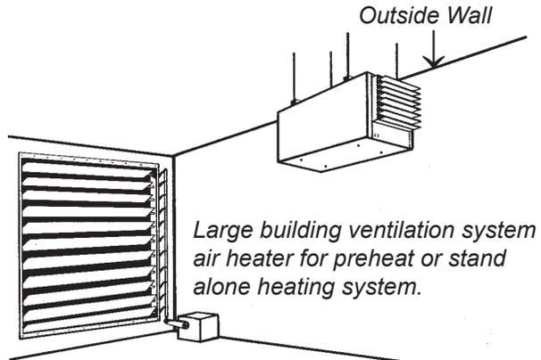
*Large building ventilation system air heater for preheat or stand alone heating system.*
