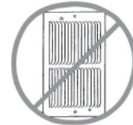
**Note: Heaters cannot be installed vertically.**
