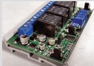
Fan Control Transducer
