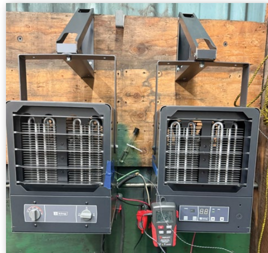
Test installation with mechanical thermostat unit and ECO2S unit mounted side-by-side.
