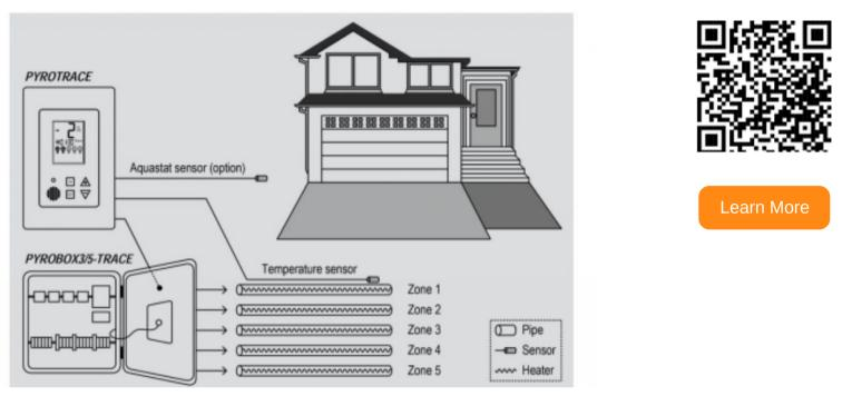
Even though self-regulating heating cables are able to adjust the amount of heat that they produce on their own, pipe trace controllers monitor the ambient temperature as it falls below the freezing point to help
