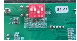
BMS Models Settings - PIR Occupancy Sensor
