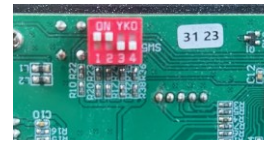
BMS Models Settings - Window/Door Sensor
