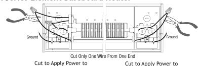
co Apply Power to Cut to Apply Power to LEFT SIDE RIGHT SIDE
