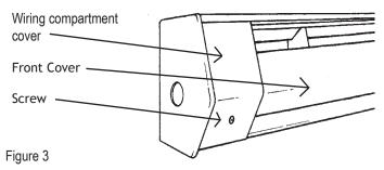
NOTE: For most efficient operation locate heaters along outside wall under windows. Position heater so it can be secured to wall stud. Power cable must enter heater through built in cable clamp or one of the knockouts provided in wiring compartment.
