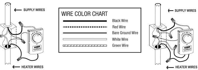
Connection Diagram for Wall Mounted Double Pole Thermostat
