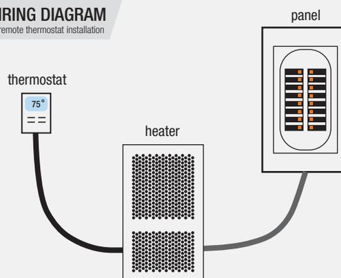
Power must be routed to heater first, then to remote thermostat.
