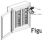
**WARNING:** Turn the electrical power OFF at the electrical panel board (circuit breaker or fuse box) and lock or tag this panel board door to prevent someone from turning on power while you are working on this heater. Failure to do so could result in serious electrical shock, burns, or possible death.
