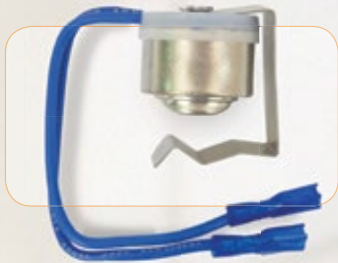
The optional aqua stat component makes sure the water temperature is over 115° before the fan is turned on.
