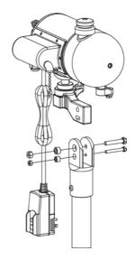
**8.** Set the rear guard in the proper position and affix it to the motor using the hex nuts, spring washers and bowl washers.
