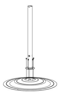
**3.** Place the upper stand pole onto the spring and press down into the lower stand pole.
