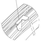
**11.** Secure the assembly on the front guard and rear guard by tightening the screw, washer and nut at the bottom of the fan guards.
