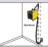
Mount bracket to wall stud and attach heater
