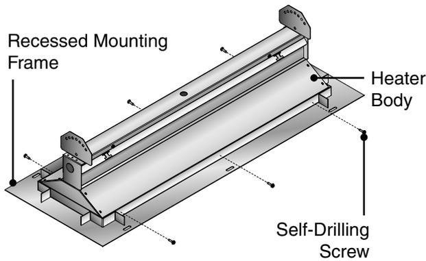
**Figure 2 • Insert into Ceiling**
