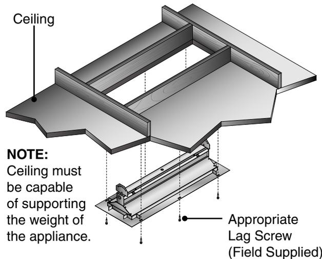
**Figure 3 • Recessed Mount - Assembled**
