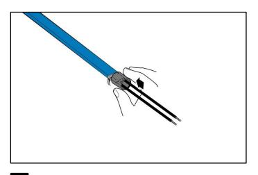
9 Place the 1/2" x 1" heat shrink tube over the cable as shown.
