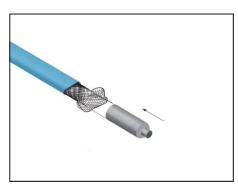
5 Push back the braid and slide the heat shrink cap over the end of the cable..
