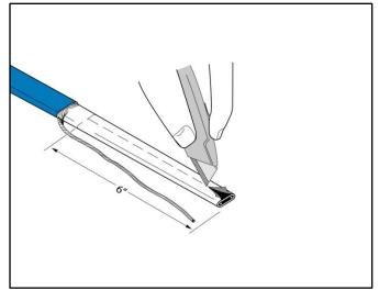
Twist and position the braid to one side of heating cable and then cut the insulating jacket back 6". Lightly score the inner insulating jacket and then bend the cable to break the jacket and peel it off.
