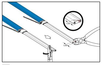
Notch the conductive core at the end and twist it back to peel the bus wires from the core.
