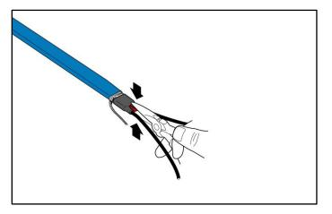
11 Immediately pinch the tube with pliers between the bus wires while it is still hot and hold for 10 seconds
