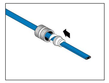
If using a weatherproof seal tight fitting (not provided with kit), slide the fitting onto the end of the cable as shown above.
