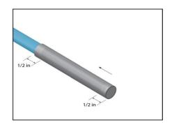
9 Slide the 5" heat shrink tube over the woven braid, allowing it to extend 1/2" past the end of the woven sleeve just applied.
