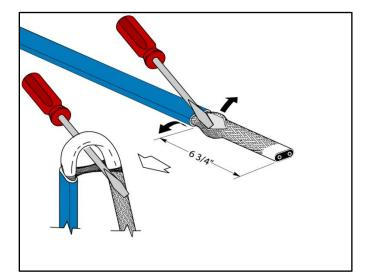
3 Cut the braid and push it back to loosen it as shown. Bend the cable and gently pull it through the braid.
