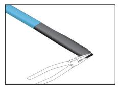
1 While the shrink tubing is still hot, gently squeeze the end with pliers and hold it until it has cooled.
