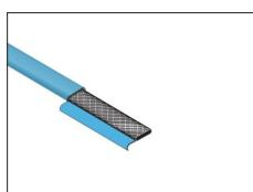
2 Remove the outer jacket to expose the braid.
