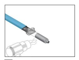
6 Apply heat evenly until the cap shrinks around the cable.
