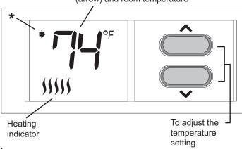
When you push one of the temperature setting buttons, a little arrow appears on the left corner of the LCD. If no other button is pushed for the next 5 seconds, the arrow will disappear and the room temperature will reappear on the LCD. To increase the temperature, press the upper button (♠) and to decrease it press (▶) the lower button.
